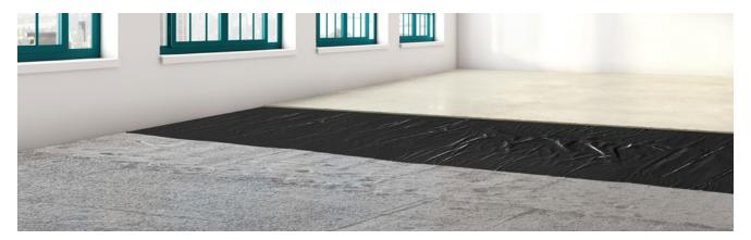
Part of the *TOPFLOW* liquid flowing screed range, *TOPFLOW* Screed A FINIO has been developed as a thin readymix screed solution with minimal thickness of 20mm (Unbonded), 25mm (resilient layer - rubber based resilient layers only) 30mm (floating insulation must be a minimum 140KPa), if not depths must be increased to 35mm domestic, 40mm commercial.
