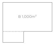
Joint required as the corner makes up over 50% of the area's length.
